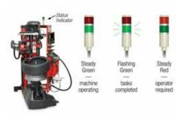
Most Technicians mount and balance assemblies sequentially by first demounting and mounting all four tires, then balancing all four assemblies. Advanced tire changers free the operator to balance assemblies while the tire machine demounts the next tire autonomously, which adds capacity and reduces the time Technicians spend on each job.
